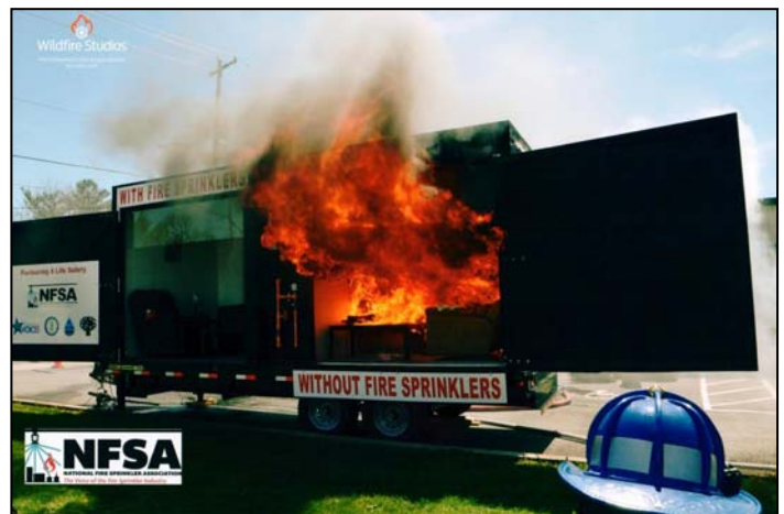
Side-by-side burn demo, just after the unsprinklered side flashed over.
